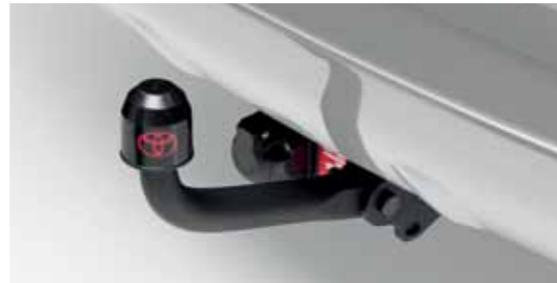
Toyota towing hitches are available with a fixed or detachable hook. Both provide a strong towing capability and will support Toyota rear mounted bicycle holders.
